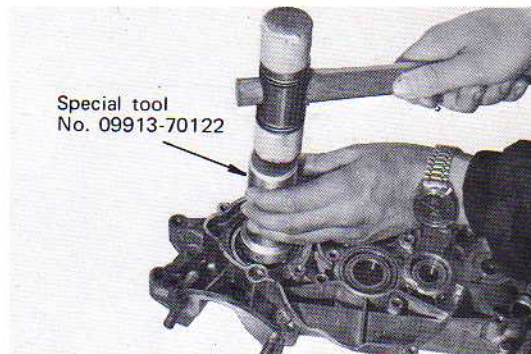
Fig. 8-61. Installing Bearing
