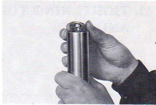
Fig. 11-2. Removing the fork inner tube cap bolt
